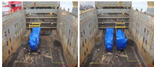
VIEW OF MAIN ENGINE UNDER LOADING IN AT AFT SECTION IN NO. 2 LOWER HOLD.
